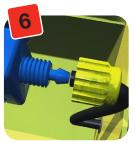
The AQUAvalve can now be connected to the 6mm pipe. Unscrew the yellow collar and push the pipe through it. Push the 6mm pipe onto the nozzle of the AQUAvalve and then replace the yellow collar by screwing it onto the AQUAvalve.
